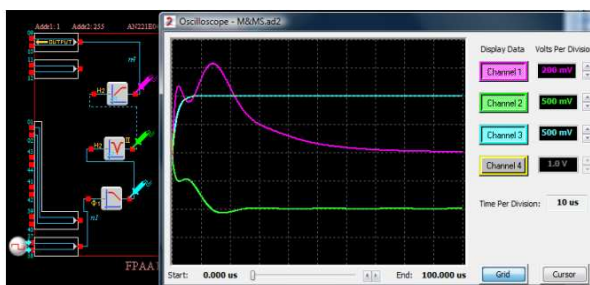
Fig. 9. Exemplary circuit built in FPAA and simulation results for nominal parameters.
